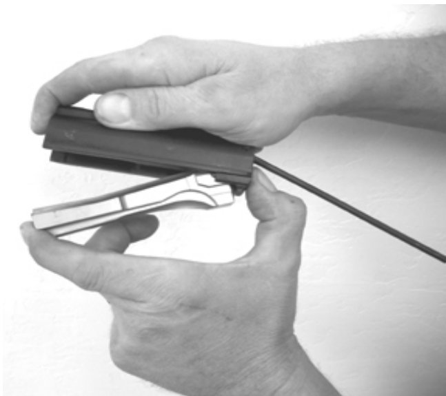
Fig. 30 Separating the Carrier from the Bolt Disengage the fore part of the bolt from the carrier and continue to separate it with a levering movement against the rear part of the bolt, keeping the thumb on the rear end of the firing pin.
