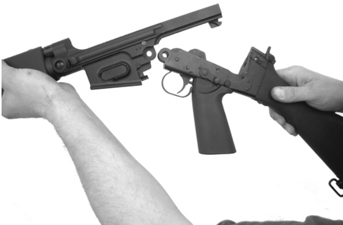
Fig. 29 Separate the Upper Assembly from the Lower Assembly Unscrew the Hinge Bolt and remove it. The Upper Assembly will separate from the Lower Assembly.
