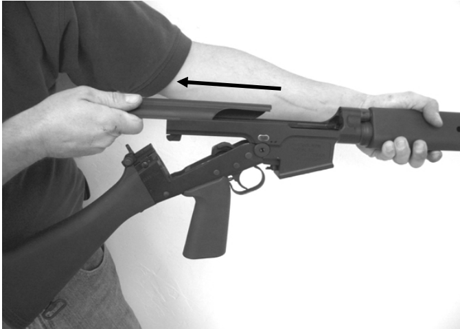
Fig. 28 Removing the Receiver Cover Slide the receiver Cover to the rear.
